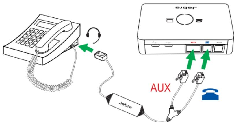
For specific instructions on connecting an electronic hook switch adapter\* to a desk phone, please refer to the cabling documentation supplied with the adapter.
