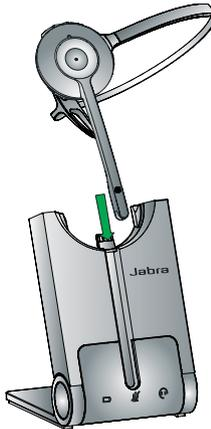
Dock the headset, as illustrated. When the primary headset is docked correctly the headset LED will be white for 5 seconds, and the headset battery will begin charging, if needed.
