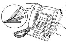
The tilt angle of the operation board can be adjusted to four step-angles.
