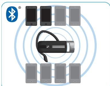
The headset can save the connection profiles of up to eight **Bluetooth** devices with which it has been paired. After switch-on, the headset automatically tries to connect to the two last connected **Bluetooth** devices. You can only connect a third **Bluetooth** device after having switched off the first or the second **Bluetooth** device.
