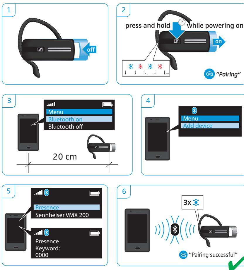
If pairing is not successful within 5 minutes, the headset automatically returns to connectable mode. Repeat the pairing procedure.
