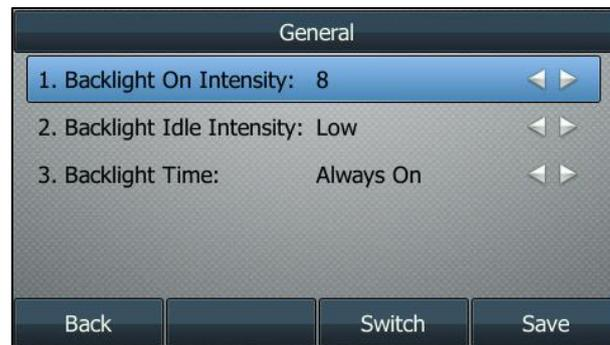
2. Press ◀ or ▶, or the **Switch** soft key to select the desired level from the **Backlight On Intensity** field.
