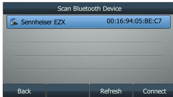
3. Select the desired Bluetooth headset and press **Connect** soft key.
