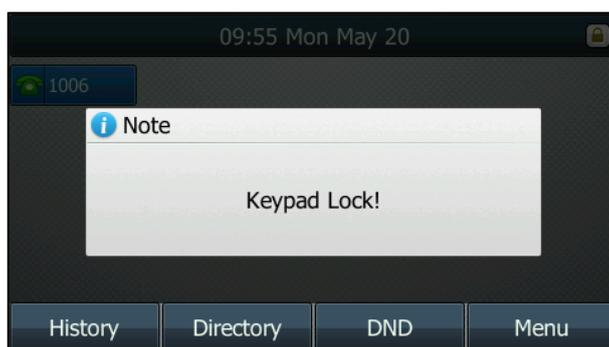
You can configure the interval (in seconds) to automatically lock the keypad instead of long pressing
